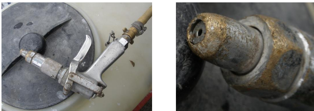
Figure 9. RIPA spray gun attached to delivery hose and close-up of nozzle at host nursery.
